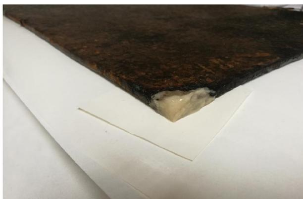
Fig. 17. The corner pasted with the pulp & CMC mixture.
