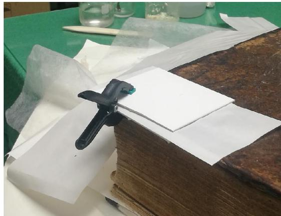
Fig. 15. Drying the consolidated corner under pressure.
