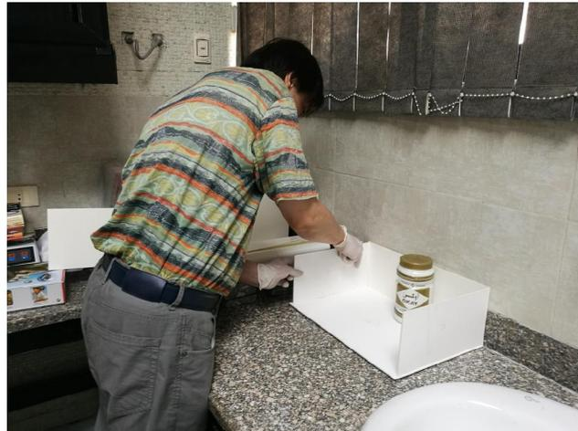
Fig. 28 (a) Assembling 4 pieces of plate into a vessel by PVAc.
